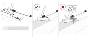
ATTENTION: In some circumstances, it is not possible to lift the boards at an angle, so they lock together (for example, underneath door frames or radiators etc.). In such cases, you can fit the pieces together with the boards flat, bearing in mind that you should *not directly strike the boards*.
